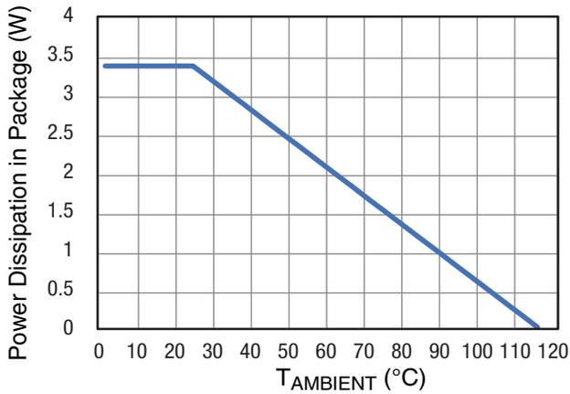
Figure 14. Package Thermal Derating
