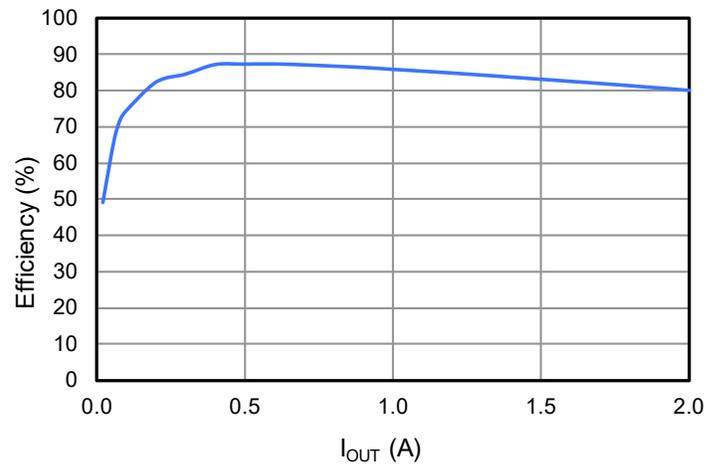
Figure 11. Efficiency Channel 2,
