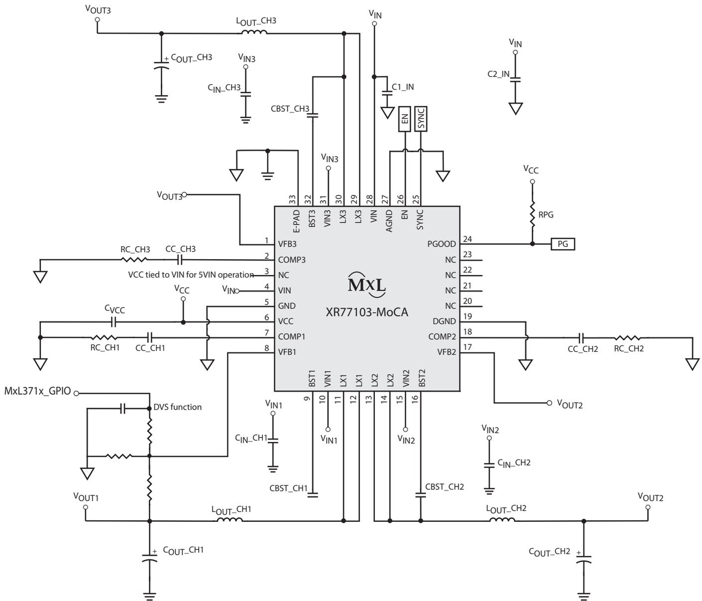
Figure 20. Typical Applications Schematic
