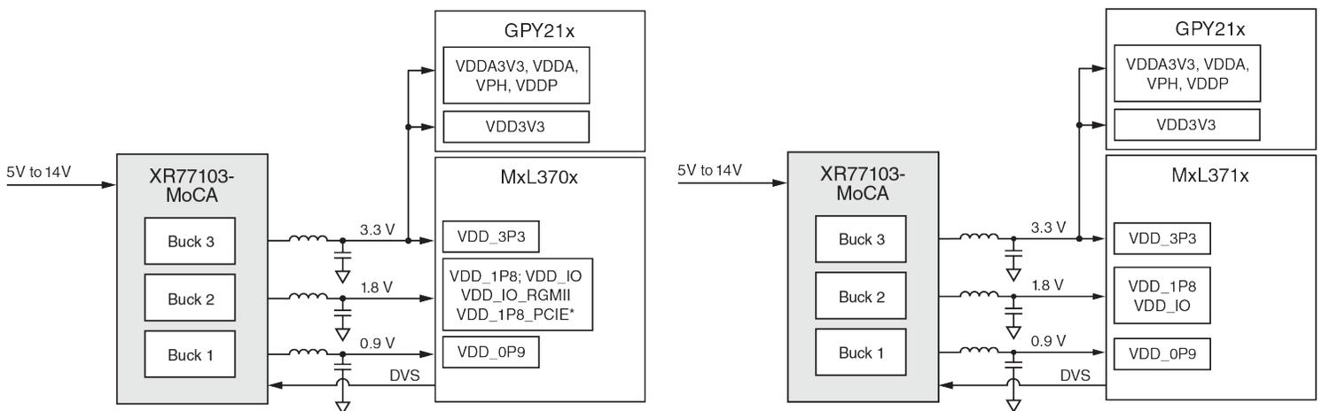
Figure 1. Power Solution for MoCA Coaxial Networking IC
