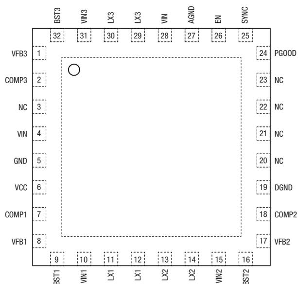
Figure 3. XR77103-MoCA Pinout
