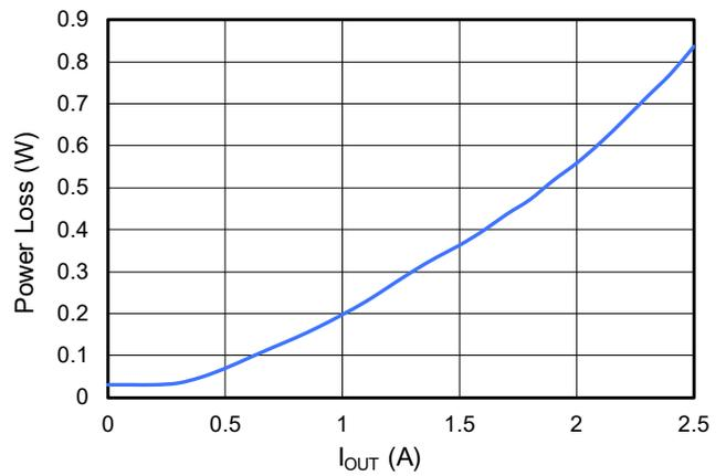
Figure 15. Channel 1 Power Loss at  $V_{IN} = 12\text{V}$ ,  $0.9V_{OUT}$ , No Airflow
