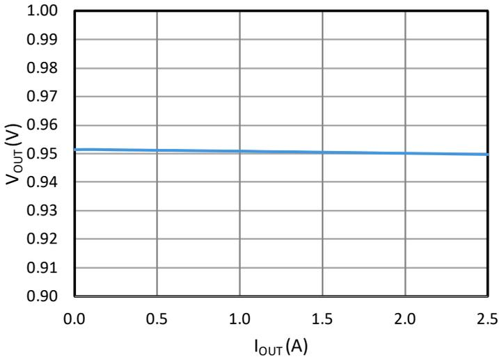
Figure 4. Load Regulation Channel 1,  $12V_{IN}$ ,  $0.9V_{OUT}$
