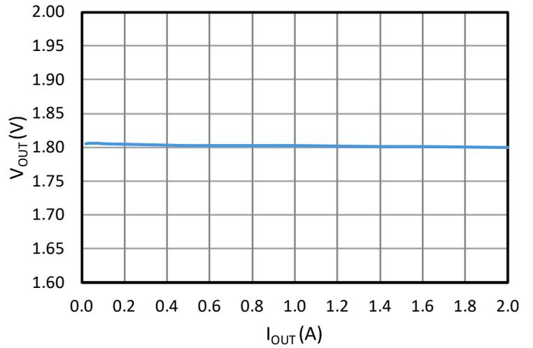
Figure 5. Load Regulation Channel 2,  $12V_{IN}$ ,  $1.8V_{OUT}$
