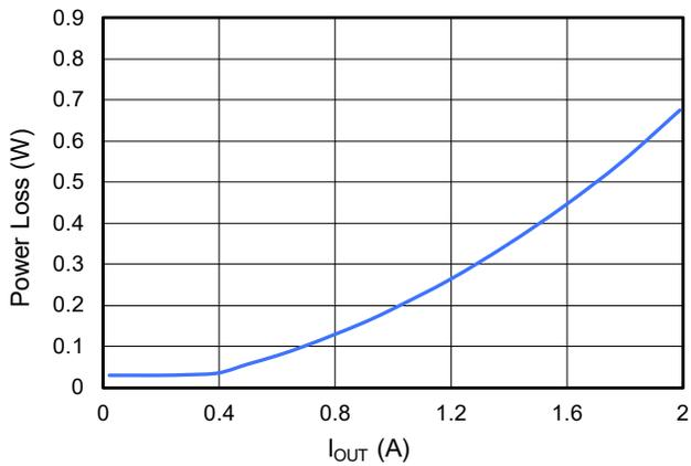
Figure 16. Channel 2 Power Loss at  $V_{IN} = 12\text{V}$ ,  $1.8V_{OUT}$ , No Airflow
