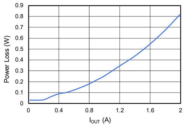
Figure 17. Channel 3 Power Loss at  $V_{IN} = 12\text{V}$ ,  $3.3V_{OUT}$ , No Airflow
