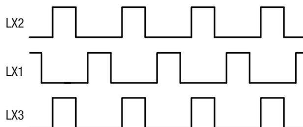
Figure 19. Out-of-Phase Operation
