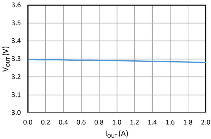
Figure 6. Load Regulation Channel 3,  $12V_{IN}$ ,  $3.3V_{OUT}$
