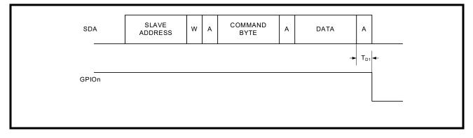
FIGURE 8. GPIO PIN INTERRUPT
